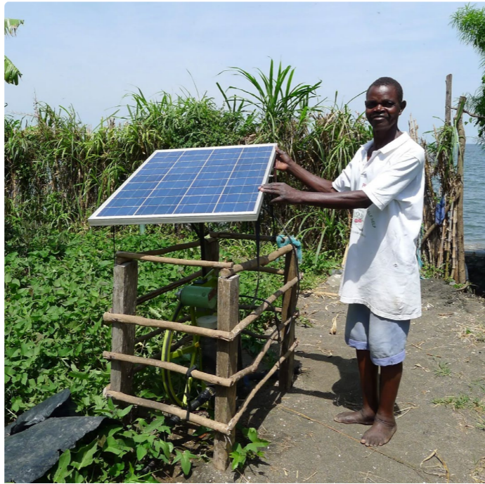
A solar panel used to power solar water pumps by Futurepump in Kenya, supported by REEEP's 10th call. Credit: Futurepump
