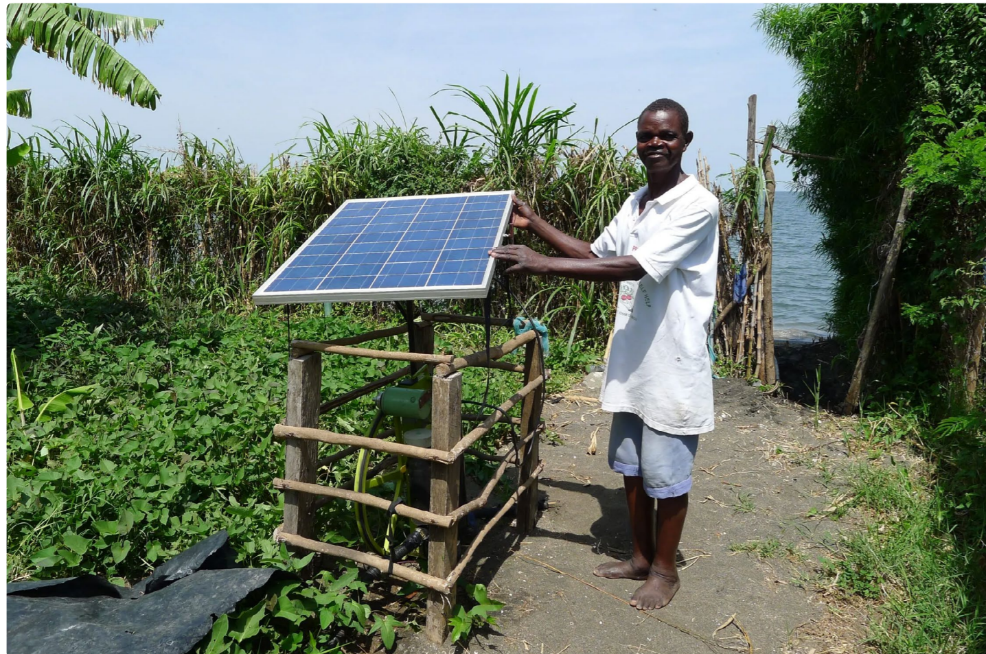
A Sunflower solar powered irrigation pump. Credit: Futurepump
